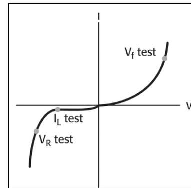
**Figure 2:** I/V curve of a typical LED.
