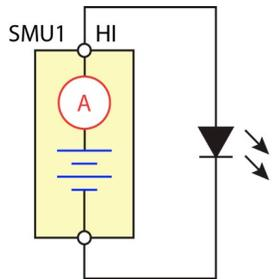
**Figure 1a:** Circuit diagram showing a SMU (Source V, Measure I configuration) in use for I/V characterization of an LED.
