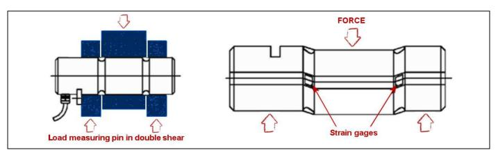
Load measuring pins are designed for many diverse applications as direct replacements for clevis or pivot pins. They have many advantages over other load sensors in that they do not normally require any change to the mechanical structure being monitored.
