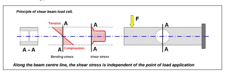
They are most commonly used in conjunction with special swivel feet and mounted in the corners of large platform scales. They are also used for vessel weighing.
