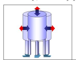
• Insulation and low thermal conductive material can be used in between the cells and the tank.
