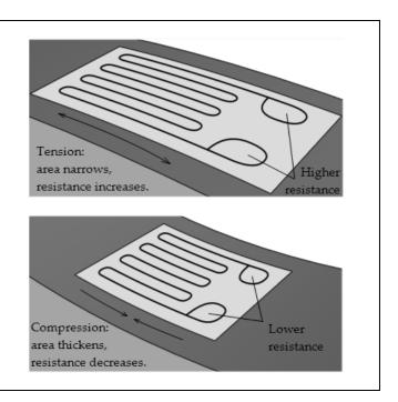
If the gages within a load cell are connected in a balanced Wheatstone Bridge circuit, and are excited by a source of AC or DC voltage, the transducer will produce an electrical output which is a direct linear function of the excitation voltage.
