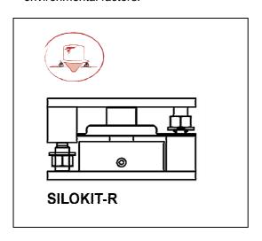
• **SILOKIT-R**: Compression low profile mounting kit including built-in stabilization plate and lift-off prevention. Designed for silo weighing.
