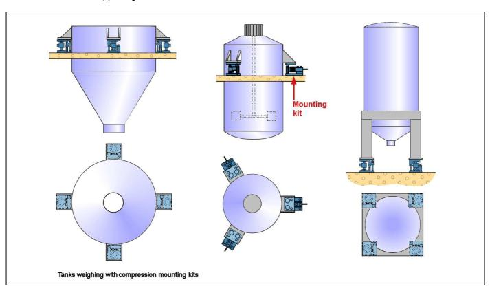
To help load cell mounting, SCAIME offers compression mounting kits especially designed for tank weighing. A typical compression mounting kit includes a top plate (which receives the load), and base plate (which is bolted to the floor or other support surface). Some kits provide also additional devices (see data sheet) as:
