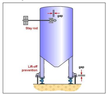
Stay rods are used to limit a tank's horizontal movement so that it will not tip or rotate. They should be positioned at or above the centre of gravity of the full tank.
