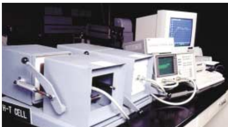
Quick and reliable fabric analysis is performed using Schlegel EMI ' TEM cell test fixtures. To ensure quality, all fabrics are routinely tested.
