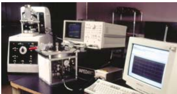
Common RF joint measurements require specialized equipment, such as the SAE ARP 1705 transfer impedance cell combined with a broadband spectrum or network analyzer.
