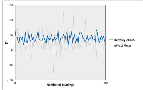
Compare the Model 2182A's DC noise performance with a nanovolt/micro-ohmmeter's. All the data shown was taken at 10 readings per second with a low thermal short applied to the input.
