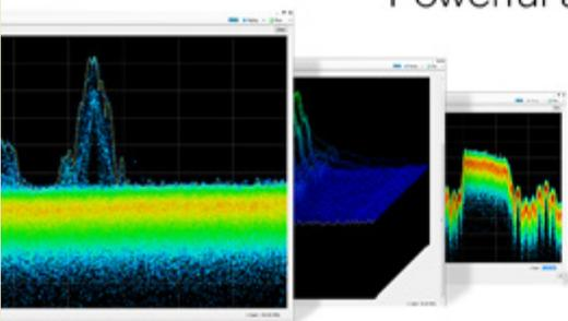
Discover the most difficult, hard-to-find events with the powerful architecture of the RSA306, featuring advanced DPX<sup>®</sup> technology to capture more data for the most accurate view of your signals.
