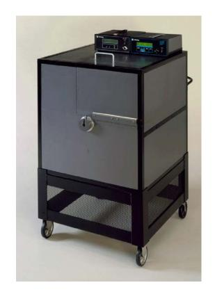
The Holaday HI-2790B Calibration Comparison System from ETS-Lindgren, complies with US Government (CDRH/FDA) requirements for evaluating calibration consistency of microwave oven survey meters used by oven manufacturers in compliance testing.
