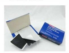
DESCRIPTION: 4000 Plyseal-V is a vinyl backed insulating mastic possessing the superior adhesive qualities and dielectric strength required to seal and insulate direct buried, submerged or overhead and electrical connections up to 1000 volts. The vinyl backing adds mechanical strength and is UV resistant. It is impervious to ozone, water, soil and corrosive chemicals 4000 Plyseal-V holds fast and permanently and will not adversly affect cable insulations and polymeric conducting shields.
