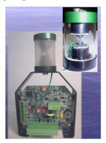
Shown above is the original RF-6/1x4 Retrofit with frosted diffuser and 2x1 SE LED engine with clear cover (inset).
