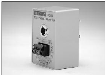
Model 8680 RTD Probe Adapter: Provides a means of connecting RTD probes terminated in either a 4-wire instrumentation connector or bare wires to safety input jacks on a 0.5 inch spacing. Use with Models 8681, 8693, 8695, or 8696.
