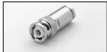
CS-631: 3-slot male triax cable mount connector for use with SC-22 cable. Mates to Models 236, 237, 238, 486, 487, 7072, and 8006.
