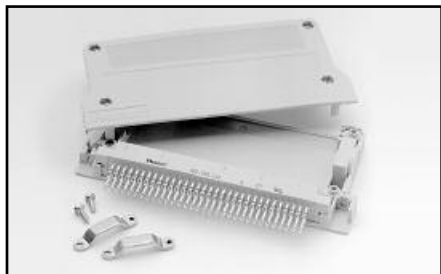
Model 7011-KIT-R: 96-pin female DIN connector with solder eyelets and strain relief. This kit can be used for assembly of custom cables to connect with the connectors on the 7011-C, 7012-C, 7013-C, 7015-C, and 7018-C switch cards. Also connects with the 7011-MTR bulkhead mount male connector.
