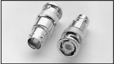
Model 6172: 2-slot male to 3-lug female triax adapter. For use in adapting Models 7065 and 2500INT inputs to 3-slot triax plugs.
