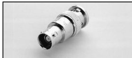
Model 237-BNC-TRX: Male BNC to 3-lug female triax adapter (guard disconnected). Terminates triax cable in BNC plug. High voltage rating for use with 237 and 7072-HV
