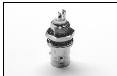
CS-630: 3-lug female triax bulkhead connector for soldered connections. Mates with CS-631.
