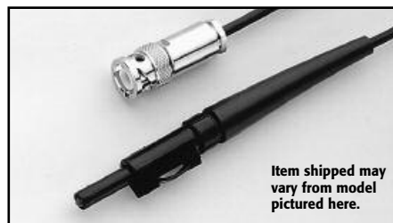
Model 237-BAN-3A Triax to Banana Plug: Triax cable center conductor terminated in a safety banana plug (guard and shield open). For connecting DMMs and other banana jack instruments to a matrix or fixture.
