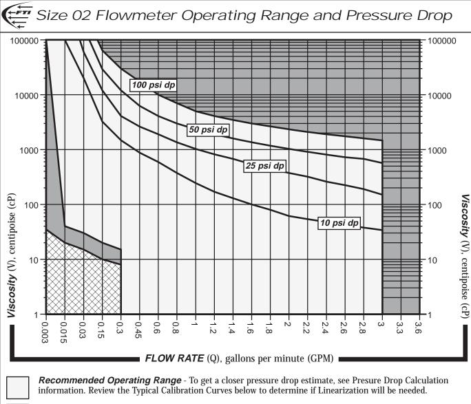
The pressure drop or differential pressure across a Flow Technology flowmeter is equal to the flow rate times a pressure drop factor. The pressure drop factor is a function of fluid viscosity and meter size. Choose the appropriate equation for the pressure drop factor, calculate it, then use it to determine the pressure drop across the flowmeter.
