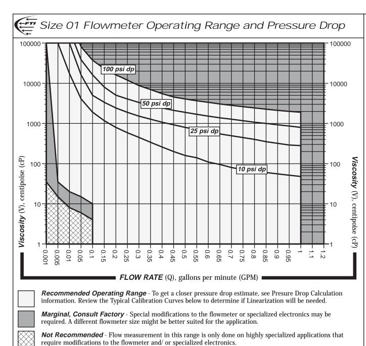
The pressure drop or differential pressure across a Flow Technology flowmeter is equal to the flow rate times a pressure drop factor. The pressure drop factor is a function of fluid viscosity and meter size. Choose the appropriate equation for the pressure drop factor, calculate it, then use it to determine the pressure drop across the flowmeter.
