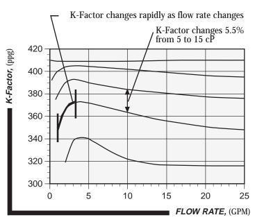
**Rapidly Changing K-Factor** - If the application is on the steeply sloped section of the calibration curve, the flowmeter size selected may be too large. A smaller size should be evaluated. In this section of the curve, the K-Factor changes rapidly as the flow rate changes. If this flowmeter size must be used, then linearization should be used. In addition, the viscosity and temperature should be closely controlled.
