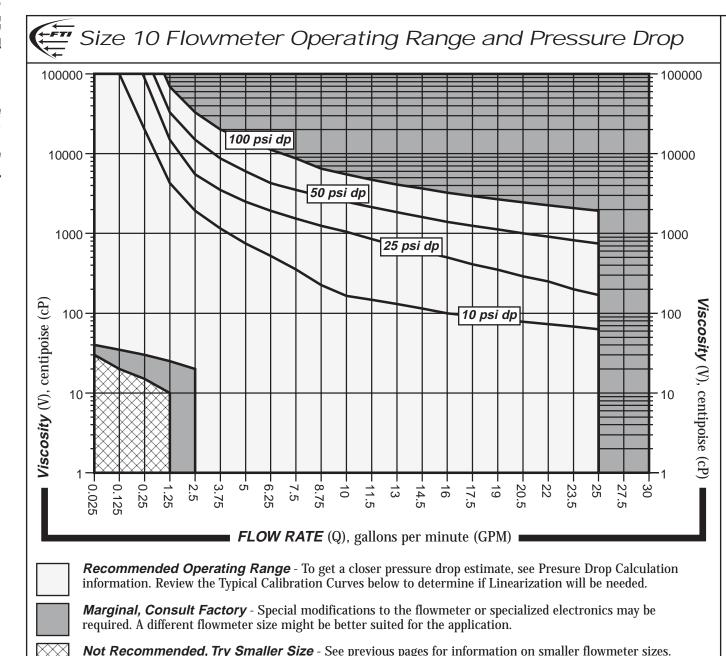
The pressure drop or differential pressure across a Flow Technology flowmeter is equal to the flow rate times a pressure drop factor. The pressure drop factor is a function of fluid viscosity and meter size. Choose the appropriate equation for the pressure drop factor, calculate it, then use it to determine the pressure drop across the flowmeter.
