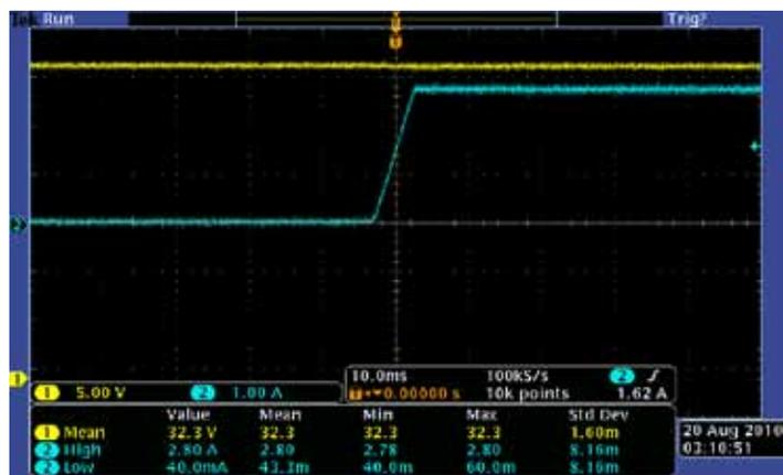
**Figure 4.** This oscilloscope screen shows the regulation of output voltage on a Keithley 2200-32-3 when the load transitions from drawing 0A to drawing 2.8A. The voltage remains stable throughout the transition.
