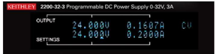
**Figure 2.** The least significant digits on the upper display correspond to the 1mV and 0.1mA readback resolution of the Keithley Series 2200 instruments. The least significant digits on the lower display correspond to the setting resolution.
