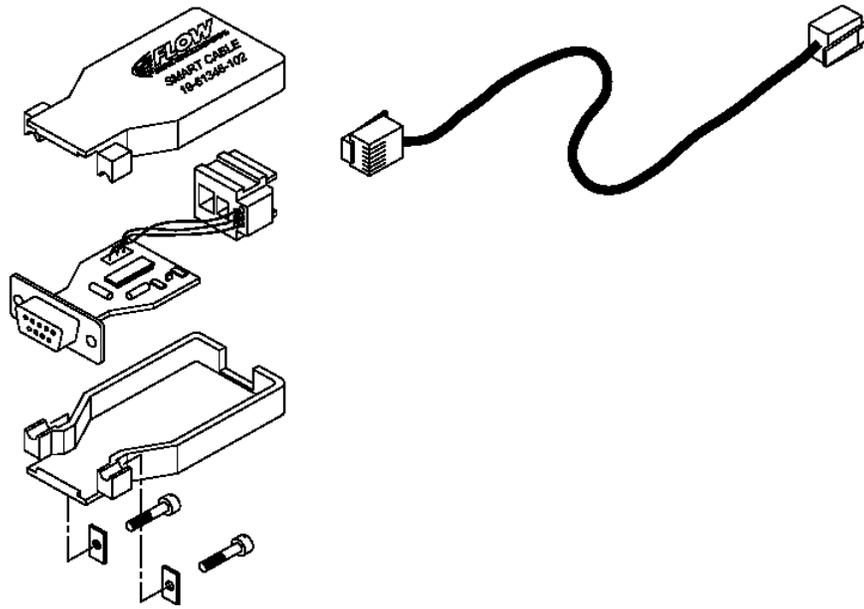
Figure 10 • LINK Interface Box with Smart Cable and RS-232 Serial Interface (P/N 19-61348-102)
