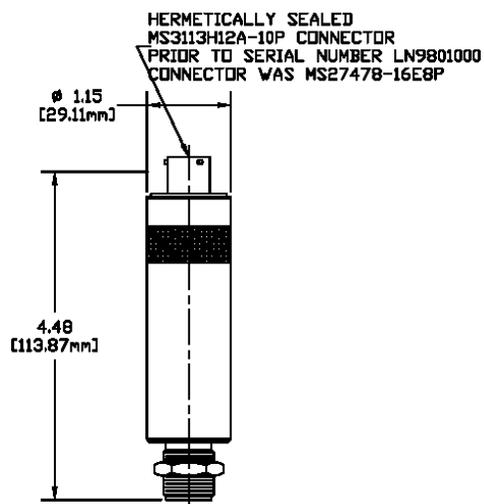
Figure 2: -1; Integral Pickoff, 10-pin MS
