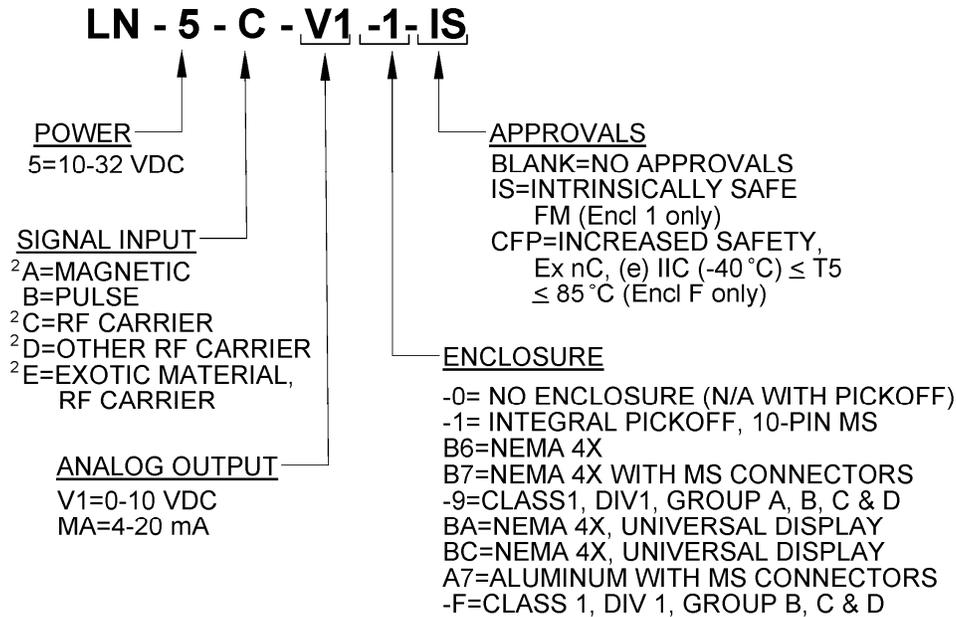
**Note:** 15-32 VDC required for 4-20 mA output configuration. Use the following formula to calculate the maximum load for loads above 550 ohms:  $R_{Load} = (Vs - 4)/.02$  At 32 VDC the maximum load is 1.4K ohms.
