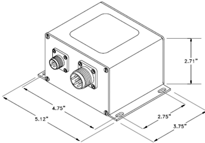
Figure 5 • A7; Aluminum Housing with MS Connectors
