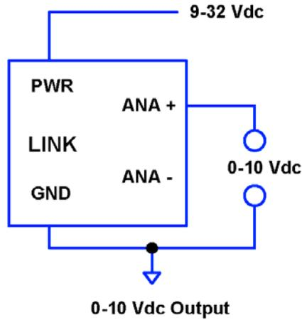
**Figure 14 • Voltage Output (MS Model Prior to 1998)**
