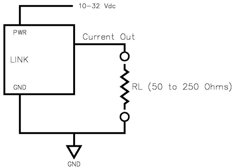
Figure 13 • Current Output, 3-Wire
