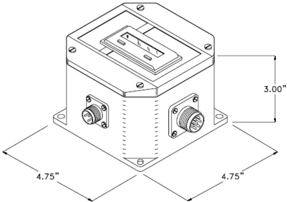
Figure 4 • B7 & BA; NEMA 4X Enclosure with MS Connectors (model with Display shown).
