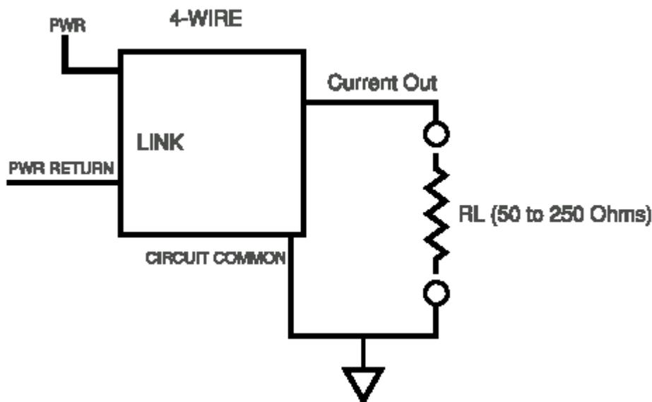
Figure 9 • Current Output, 4-Wire
