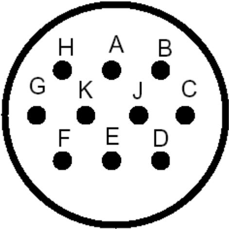
Figure 7 • Face view of 10-pin insert shown.
