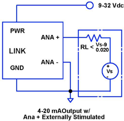
Figure 16 • Current Output - Option 2 (MS Model Prior to 1998)
