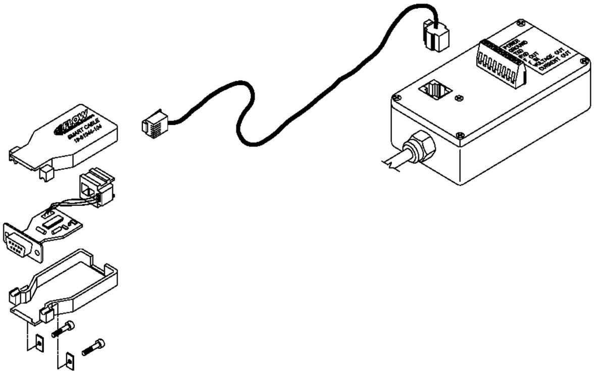
Figure 11 • LINK Interface Box with MS Connector Cable (P/N 19-61348-104)
