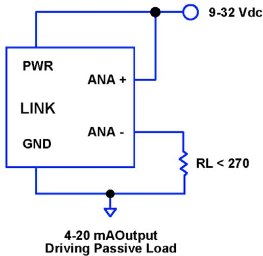
**Figure 15 • Current Output - Option 1 (MS Model Prior to 1998)**
