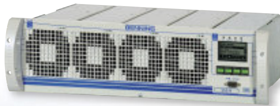
Fig. 2: 19" modular rectifier shelf with 4 modules TEBECHOP 3000 I and remote monitoring unit MCU 2500 output voltage 110 V, output current 80 A
