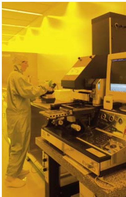
Photolithography: generating the structure on the substrate
