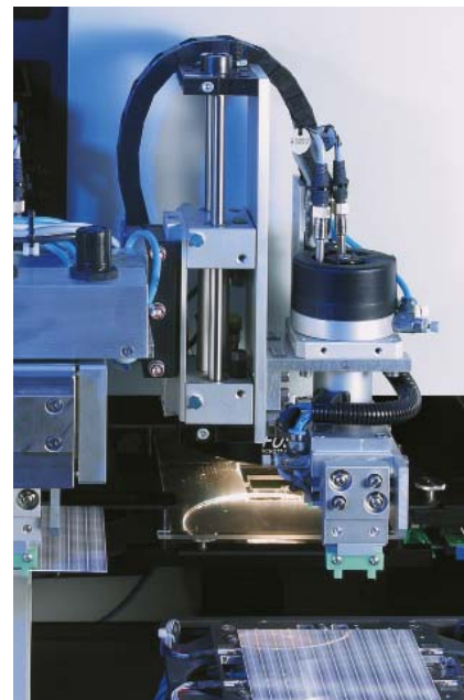
Laser calibration of platinum chip temperature sensors
