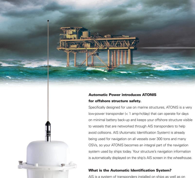
AIS is a system of transponders installed on ships as well as on Aids-to-Navigation such as buoys and markers—any offshore structure that could pose an obstacle to navigation. Ships equipped with transponders autonomously pass navigational information to each other using a common data format. The system is self-organizing and requires no operator intervention.
