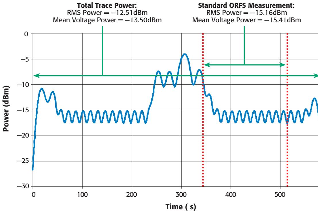
Figure 1. Zero-Span Trace
