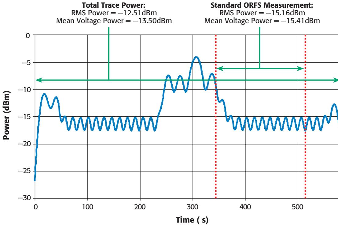
Figure 1. Zero-Span Trace
