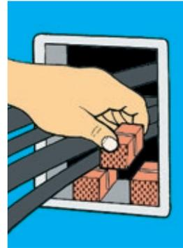
**4** When packing the transit, ensure all the insert blocks have "E" marking facing the installet.
