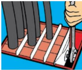
**5** Pack the frame. Tighten the bolt in the compression plate anticlockwise until there is a gap of 32-33 mm (1.26"-1.30") between the top of the plate and the inside of the frame.
