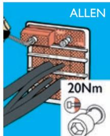
**7** Insert the final row of E-blocks. Tighten the nuts in the E-PTG to the end or 20 Nm.
