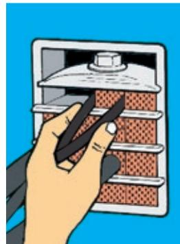
**7** Tweezers can be used, if required to aid installation of the last row of E-blocks.
