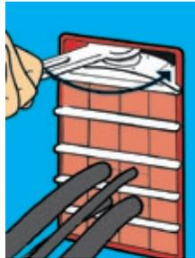
**6** Tighten the bolt in the compression plate anticlockwise until there is a gap of 32-33 mm (1.26-1.30'') between the top of the plate and the inside of the frame.
