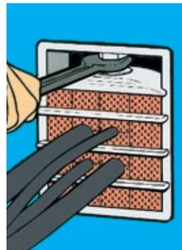
**8** Tighten the bolt in the compression plate anticlockwise until there is a gap of 32-33 mm (1.26, 1.30 ") between the top of the plate and the inside of the frame.
