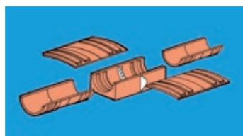
4. Attach the two inserts into the locating ridges.
