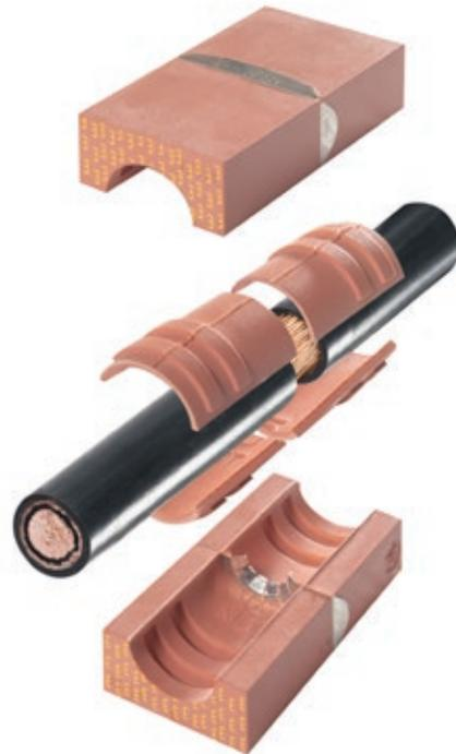
There are eleven different sizes of E-AddBlock. By tearing off the wing-like inserts, which are of varying thickness, and inserting them in the main block it is possible to accommodate 66 different cable and pipe dimensions, from 3.5 mm (0.14") to 69.5 mm (2.74"). The inserts are fitted with a locating ridge that fits exactly into furrows in the main block. These stop the block from "telescoping".
