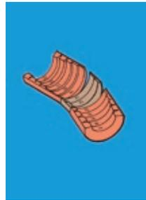
If the insert gets longer than the block, remove the current rings in the middle.
