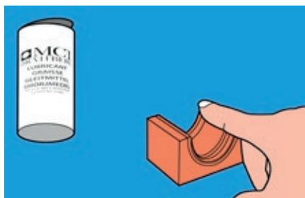
5. Lubricate carefully the inner and outer edges of the prepared RFCS module together with PTG 40 wedge and inner edge of the frame.
