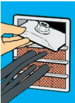
**6** Before the final row of E-blocks, the compression plate is installed. Alternatively, the E-PTG Presswedge can be fitted.
