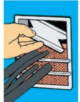
**5** Position the stayplates between each layer of insert blocks.
