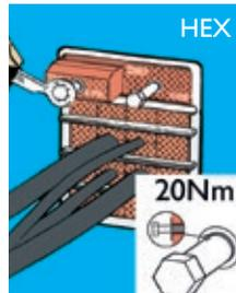
**8** Insert the final row of E-blocks. Tighten the nuts in the E-PTG to the end or 20 Nm.
