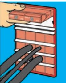
**4** Place the last two stayplates in the frame before the last row of blocks. Then fit the PTG presswedge over the stayplates.
