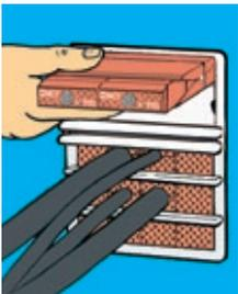
**6** Place the last two stayplates in the frame before the last row of blocks. Then fit the E-PTG presswedge over the stayplates.
