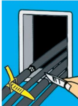
**2** Pull cables to final position. Mark cable 30 mm (1.18") from front edge of frame. Remove cable sheath 5 mm (0.2") on either side of the line.
