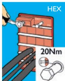
**6** Insert the final row of blocks. Tighten the nuts in the PTG to the end or 20 Nm.
