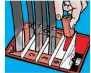
**4** Insert the outer blocks first (A, B, C, etc). Then insert the rest of the blocks. Note: block A must be rotated 90°, see diagram.
