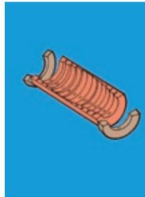
Select the two compression rings closest to the cable diameter. Remove all compression rings smaller than the selected.
