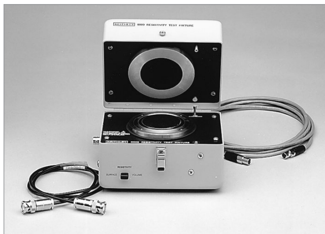
8009 Resistivity Test Fixture is compliant with American Society for Testing and Materials (ASTM) Standard D257 Standard Test Methods for DC Resistance or Conductance of Insulating Materials. The 8009 combined with the 6517B provides a complete system for making high quality, safe resistivity measurements. The 8009 comes with the 6517B-ILC-3 Safety Interlock Cable, the 7078-TRX-3 Triax-Triax Cable, and the 8607 1 kV Source Voltage Banana Jack Cable Set.
