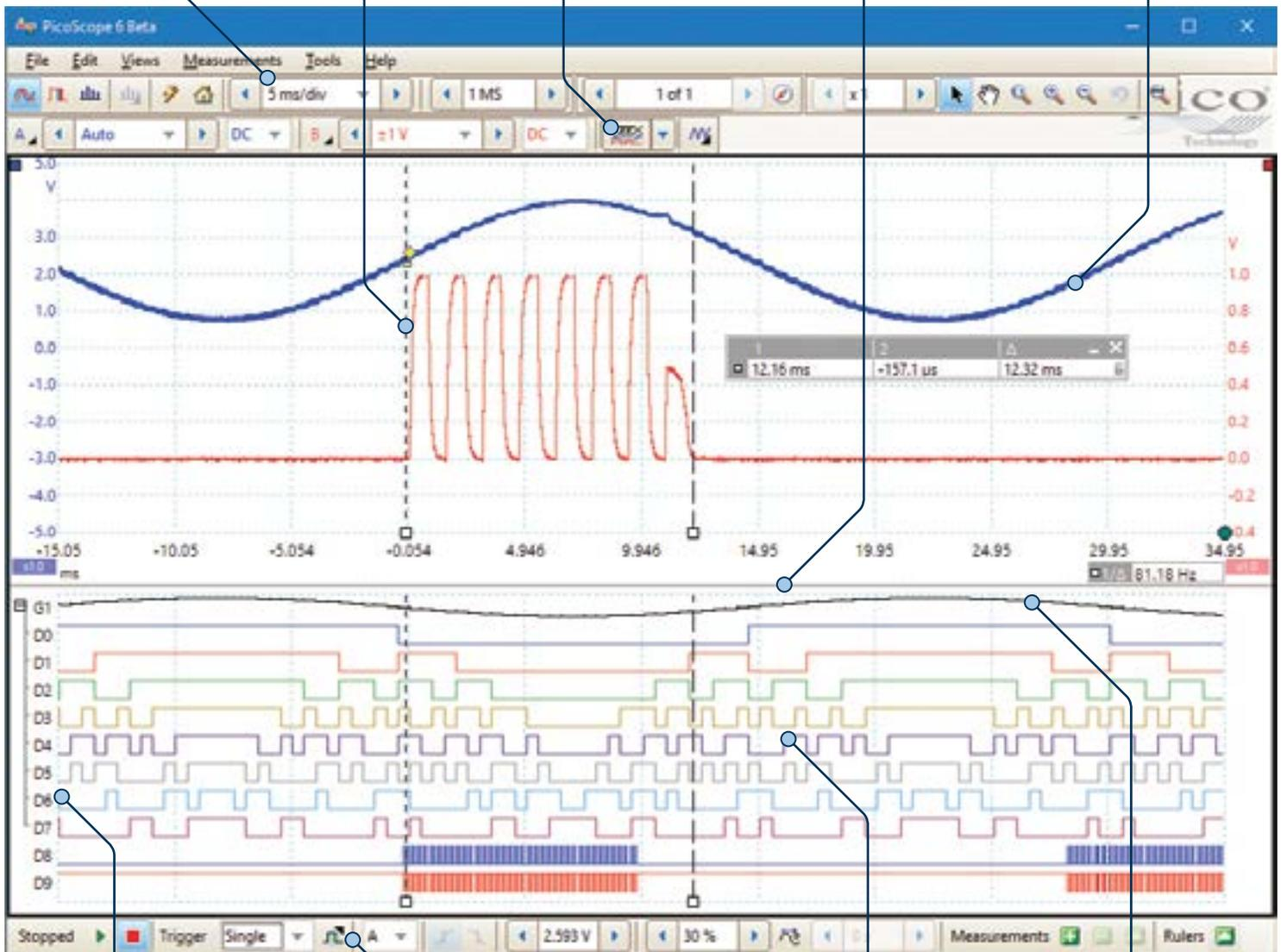
**Rename:** The digital channels and groups can be renamed. Groups can be expanded or collapsed in the digital view.
