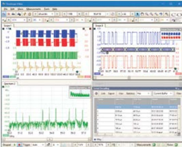
The PicoScope 6 software takes advantage of the display size and resolution and processing power of your PC – in this case displaying four analog signals, a zoomed view of two of the signals (undergoing serial decoding), and a spectrum view of a third, all at the same time. Unlike a conventional benchtop oscilloscope, the size of the display is limited only by the size of your computer monitor. The software is also easy to use on touch-screen devices – you can pinch to zoom and drag to scroll.
