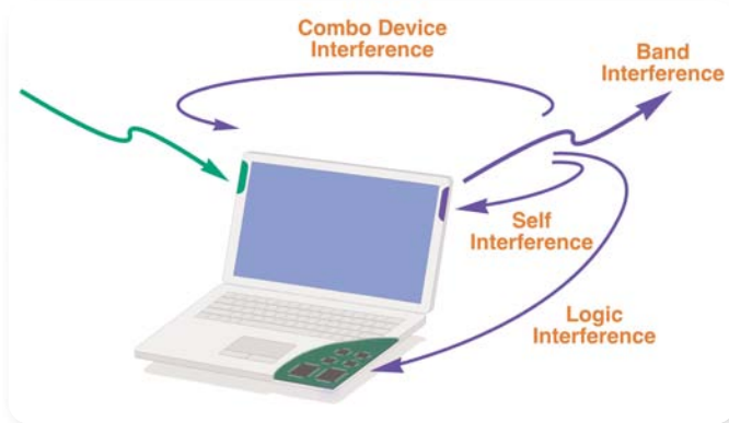
► Figure 7. Modes of combo device interference.
