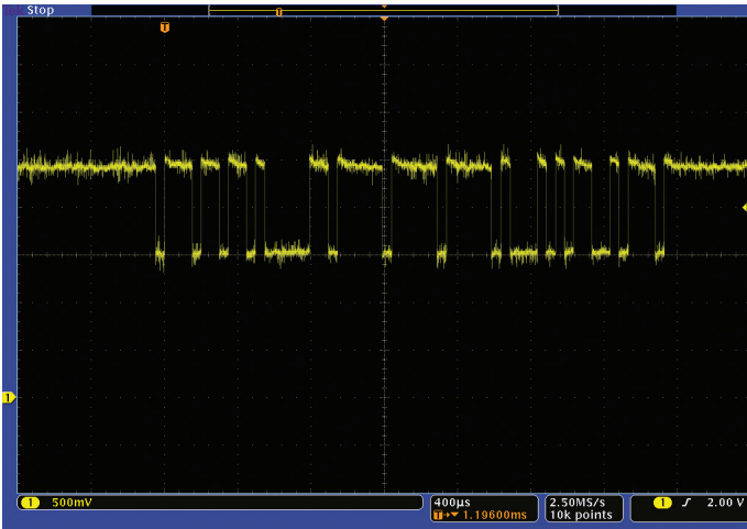
Figure 2. One message acquired from a CAN bus.
