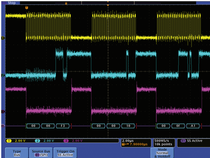
Figure 13. Correct synthesizer configuration messages.
