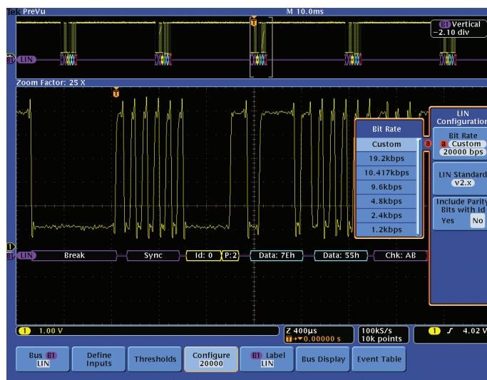
Figure 35. LIN bus setup menu and decoded frame.
