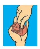
Select a suitable InsertBlock or AddBlock for the small cable. Then create a base using U-Blocks. The external measurements should be the same as the previous block.
