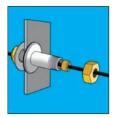
O Size the second washer to the cable and insert it to the cable if required
