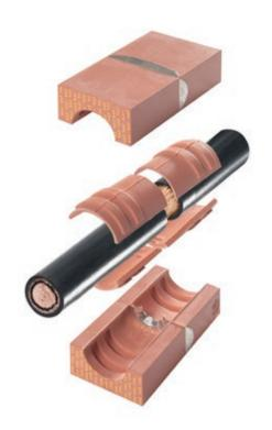
There are eleven different sizes of E-AddBlock. By tearing off the wing-like inserts, which are of varying thickness, and inserting them in the main block it is possible to accommodate 66 different cable and pipe dimensions, from 3.5 mm (0.14") to 69.5 mm (2.74"). The inserts are fitted with a locating ridge that fits exactly into furrows in the main block. These stop the block from "telescoping".
