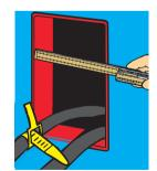
Measure the opening and check that the measurement is within the tolerance range I 20.5 mm +/- 0.5 mm (4.74"+/-0.02"). Check that the frame is clean and pull through the cables. Measure the diameter of the cables and choose suitable blocks. Lubricate the inner faces of the frame.
