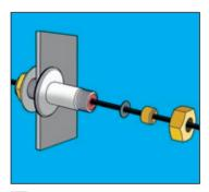
**9** Carefully push complete seal and cable back into gland maintaning EMC contact.
