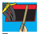
Measure the opening and check that the measurement is within the tolerance range 120.5 mm +/- 0.5 mm (4.74"+/-0.02"). Check that the frame is clean and pull through the cables. Measure the diameter of the cables and choose suitable blocks. Lubricate the inner faces of the frame.
