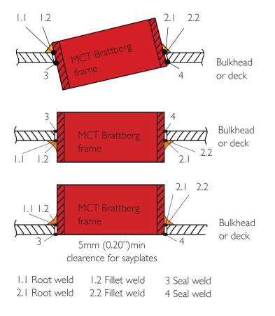
Fillet weld size for a centre-placed frame
