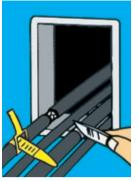
Pull cables to final position. Mark cable 30 mm (1.18") from front edge of frame. Remove cable sheat 5 mm (0.2") on either side of the line.
