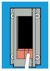
2. Mount the Alf frame to your cabinet with the supplied bolts and with the gasket in between the flange and the cabinet.
