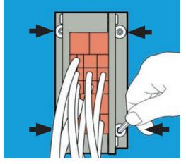
6. Finally tighten the four mounting bolts against the cabinet.
