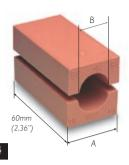
InsertBlock. The blocks are identified by their width (A) and hole diameter (B). A block that is 30 mm (1.18") wide and has a hole diameter of 18 mm (0,71") is marked 30/18. This marking is cast into the block.
