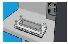
2. Install the frame and gasket directly on the cabinet cutout before installing the cables.
