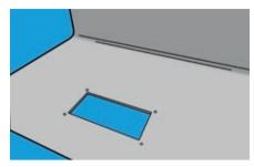
I. Start the installation by ensuring that the cutout made in cabinet correspond to the cutout pattern in the installation manual.
