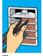
Tweezers can be used, if required to aid installation of the last row of E-blocks.
