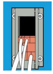
4. Fill up the frame with cables, insert blocks and spare blocks.
