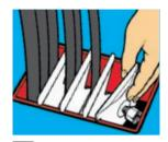
To prevent the blocks from falling through during horizontal installation, fit all the stayplates and the compression plate first. Check the RG plan to make sure the cables are positioned correctly.
