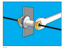
8 Push cable trough assembled gland and tighten nut.
