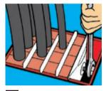
Pack the frame. Tighten the bolt in the compression plate anticlockwise until there is a gap of 32-33 mm (1.26"-1.30") between the top of the plate and the inside of the frame.
