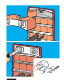
7 Insert the STG endpacking with the tongue around the compression bolt. Tighten the nuts in the endpacking until 12-15 mm (0.47-0.59") of thread is visible.
