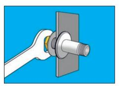
3 Tighten the lock nut.
