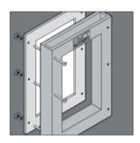
1. Fix frame to opening using gasket and M6 screws supplied.
