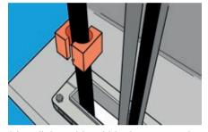
6. Install the cable within the prepared halves of RFCS module.
