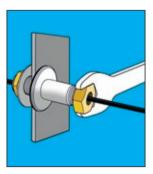
Push cable trough assembled gland and tighten nut.
