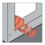
5. Detach sealing rings from main block and retain ring corresponding to measured cable size. In this example 26 mm (1.02")
