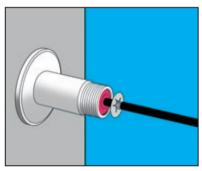
6 Slide EMC piece over cable until contacts with cable braid.
