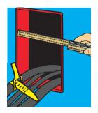
Measure the opening and check that the measurement is within the tolerance range 120.5 mm +/- 0.5 mm (4.74"+/-0.02"). Check that the frame is clean and pull through the cables. Measure the diameter of the cables and choose suitable blocks. Lubricate the inner faces of the frame.
