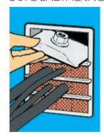
Before the final row of E-blocks, the compression plate is installed. Alternatively, the E-PTG Presswedge can be fitted.
