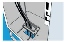
15. Install the preterminated cables between the two halves of RFCS frame.
