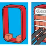
Begin packing with the special corner blocks. Proceed as shown in image 3 and then see STG Endpacking image 4-6. Insert endpacking C-STG (with special corner blocks). Tighten the nuts on the endpacking to compress and complete the seal. About 12 mm (0.47") of the thread should protrude on each bolt.
