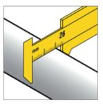
2. Measure cable. In this example cable has a diameter of 26 mm (1.02").
