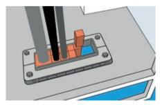
20. Remove all the unprepared CS modules from the frame.
