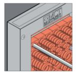
10. Build up the frame and repeat the process described in steps 2-9. In this example 2 more cables have been added using other block sizes.
