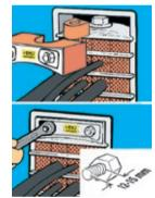
Insert the E-STG endbacking with the tongue around the compression bolt. Tighten the nuts in the endpacking until 12-15 mm (0.47-0.59") of thread is visible.
