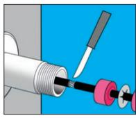
Pull cable though gland and carefully trim 5 mm of outer sheath.
