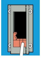
3 Do not tighten the mounting bolts too much, the frame / flange should still be able to slide underneath the bolt head.
