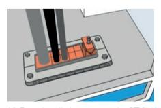
19. For reinstallation remove the PTG 40 wedge.
