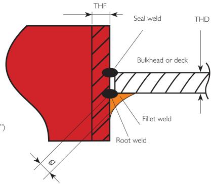
Maximum allowable root gap for fillet joint
