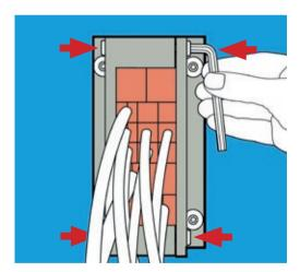
5. Tighten the two compression bolts until the cables are not movable
