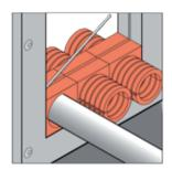
9. If more cables are required repeat the sequence. If not insert blanks to complete row and insert staybar to secure.
