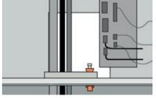
I I-I2. Tighten the PTG 40 wedge until it is almost even with the frame surface to obtain IP 65/67 rating.
