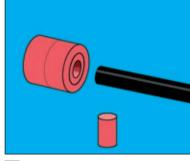
4 Remove the minimum number of rings to allow cable to pass though the seal.
