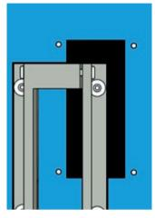
I. Drill hole pattern and cut out for the frame according to table and sketch.
