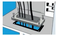
18. Fix the RFCS frame together with back gasket on the cabinet cutout by tightening with mounting hardware.
