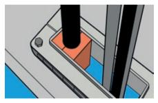
7. Install the RFCS module together with cable from the front until the module rests against the back wall of the frame
