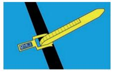
3. Use the cable selector to find the exact diameter of cable by wrapping around the circumference of cable.
