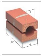
The E-Blocks are identified by their width (A) and hole diameter all the insert blocks have "E (B). A block that is 30 mm (1.18") marking facing the installet. wide and has a hole diameter of 18 mm (0.71") is marked 30/18. This marking is cast into the block
