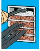
Tighten the bolt in the compression plate anticlockwise until there is a gap of 32-33 mm (1.26, 1.30 ") between the top of the plate and the inside of the
